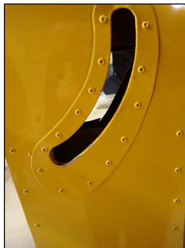
Photo No. 6 and Photo No. 7 : Damage to reinforced slot for flaperon mechanism
