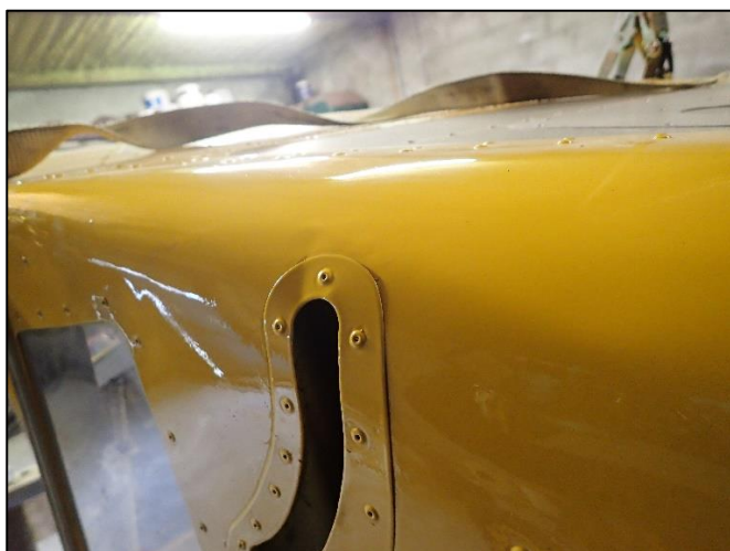
Photo No. 6 and Photo No. 7 : Damage to reinforced slot for flaperon mechanism
