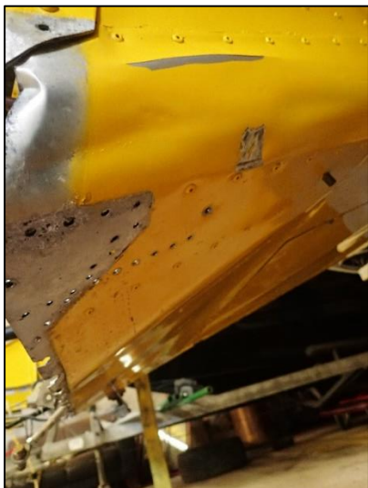
Photo No. 4 and Photo No. 5 : Wrinkling of aircraft skin
